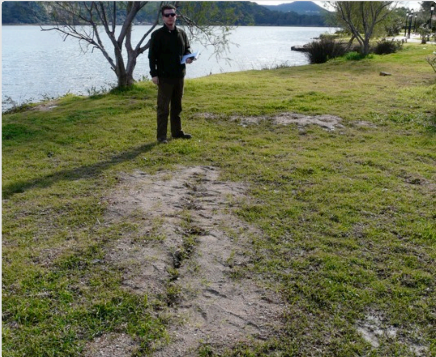
Figure 6. Liquefaction phenomena in the waterfront area in Argostoli (photo taken on 8/02/2014)
